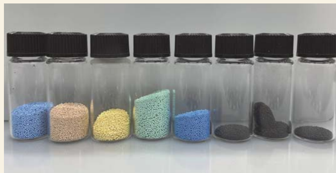
Fig. 3. Carbon-supported metal catalysts and their precursors before carbonization.
