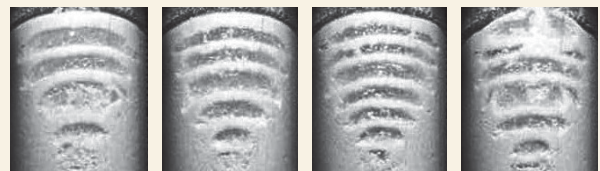
Fig. 2. The multilayered structure of bubbles generated in a fine powder bed oscillates horizontally with a small amplitude.
