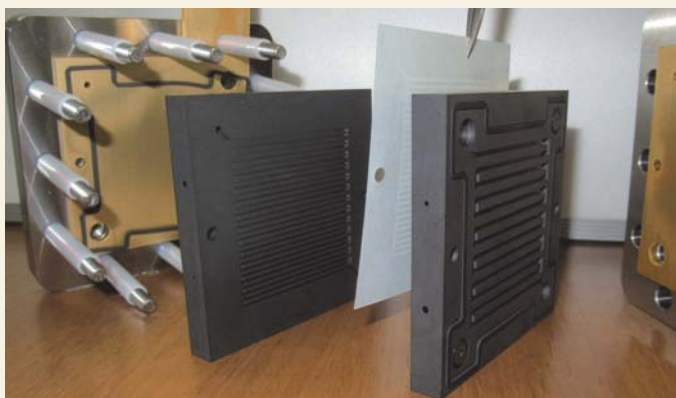
Fig. 2. A laboratory-scale polymer electrolyte fuel cell equipped with cooling channels.
