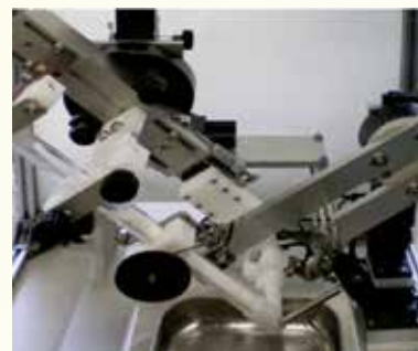
Fig. 3. Micro-feeding of nanoparticles based on vibration shear flow.
