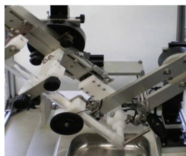
Fig. 3. Micro-feeding of nanoparticles based on a novel shear vibration method.
