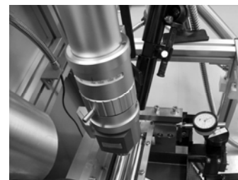
Fig. 4. Microscopic observation of particle behavior through a high-speed camera (120,000 fps).
