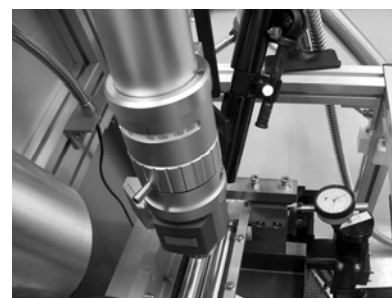
Fig. 3. Microscopic observation of particle behavior through a high-speed camera (120,000 fps).
