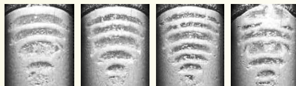
Fig. 2. Multilayered structure of bubbles generated in a fine powder bed oscillating horizontally with small amplitude.
