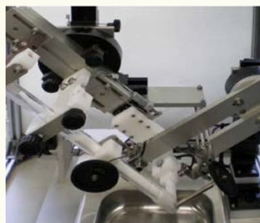
Fig. 3. Micro-feeding of nanoparticles based on vibration shear flow.
